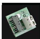
Platine IN (Einspeiseplatine) PCB IN (Supply PCB)
